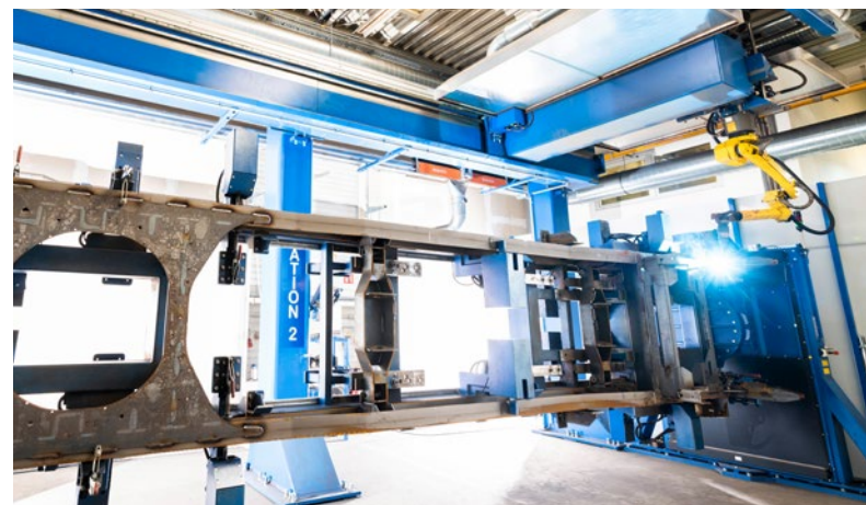
The positioner has set the chassis upright, while the robot is welding in the flat position.
