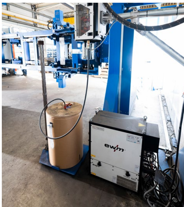
The Phoenix puls welding machine with drum feed via a drive 4X wire feeder.
